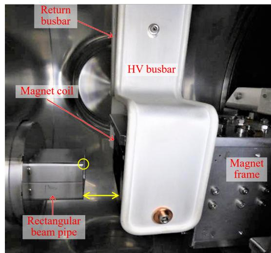
Figure 3: Photo of inside of one end of an MKBV tank.
