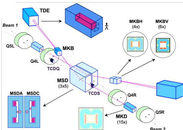
Figure 1: Schematic overview of the LHC extraction area.
