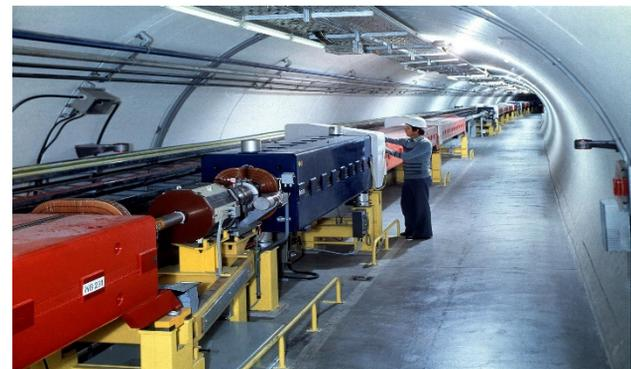
Figure 2: View of a SPS' arc with quadrupole (red), dipole (blue) magnets, and the interposed short straight sections. The latter must be removed to have access for the coating of the magnet's vacuum chambers.
