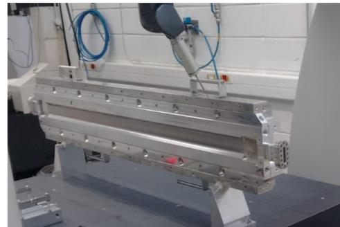
Figure 6: CMM measuring process.
