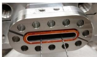
Figure 8: The two cathodes approximate position.
