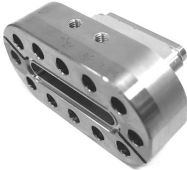
Figure 3: In-house diffusion bonded bimetallic flange.
