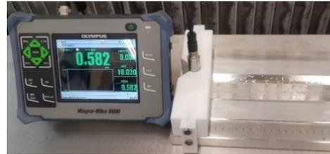
Figure 5: Prototype under measurement with the Magna Mike 8600.
