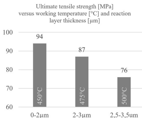
Figure 5: Joints tensile strength vs working temperatures.
