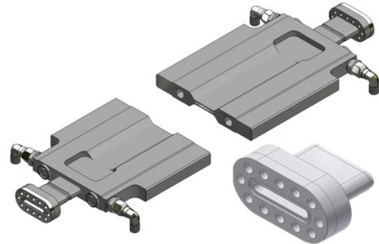
Figure 1: Virtual design of undulator and bimetallic flange.
