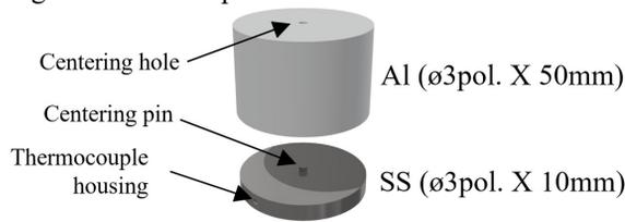
Figure 3: Virtual design of Al and SS parts.
