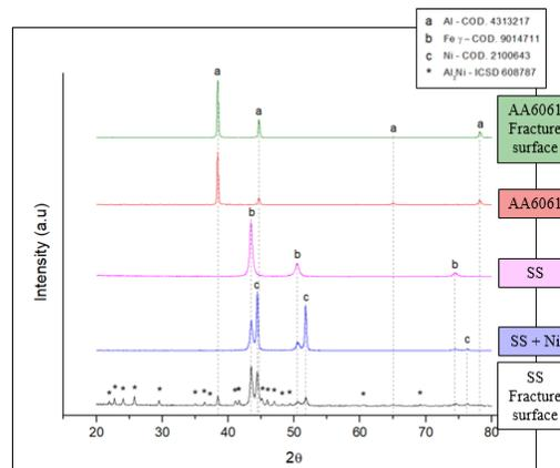
Figure 6: Diffractogram of Al and SS fracture surfaces.
