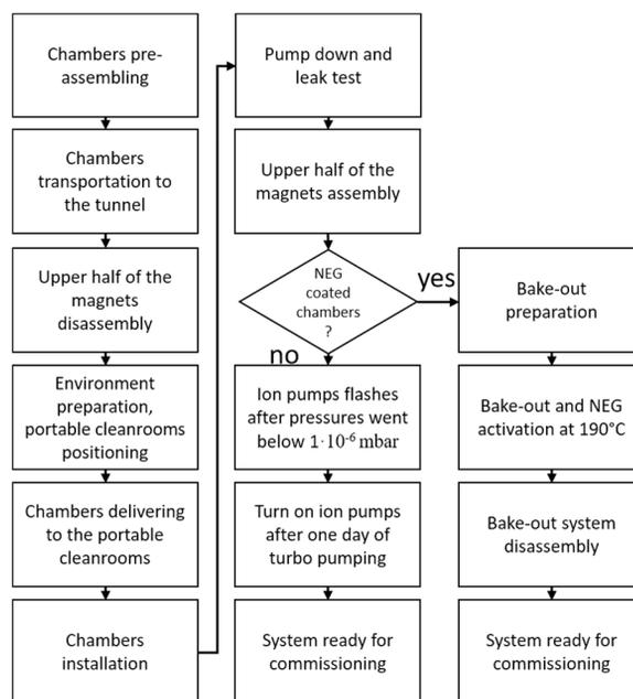
Figure 1: Vacuum installation process flow chart.
