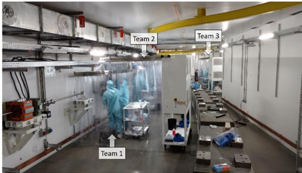
Figure 2: Vacuum teams assembling the booster sectors.
