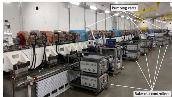
Figure 4: A storage ring arc ready for the bake-out process.
