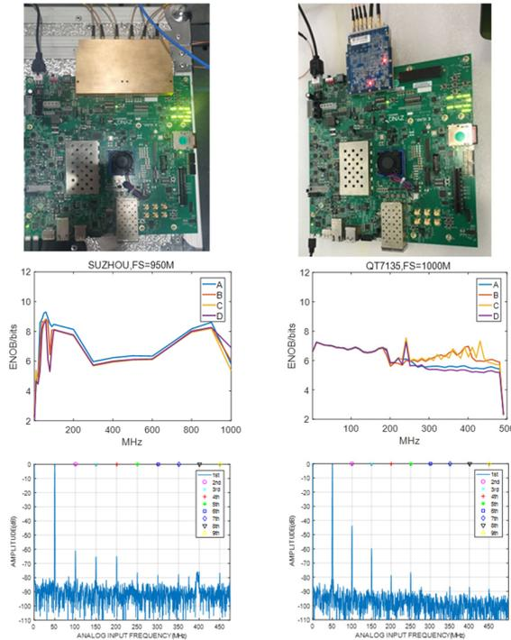
Figure 1: Lab evaluation of domestic(left) and abroad(right) ADCs.
