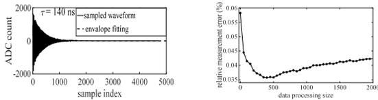
Figure 7: Sampled cavity BPM signal waveform(left) and relative resolution VS. data processing size(right).
