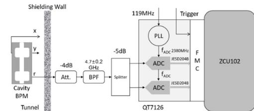
Figure 6: Test block diagram of RF processor.
