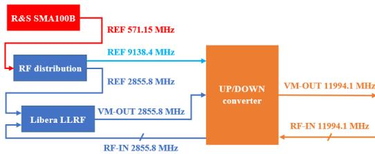
Figure 3: Block diagram of TEX LLRF system.
