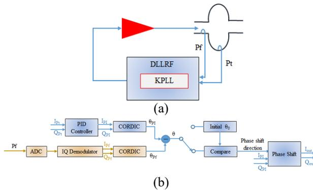
Figure 3: (a) The simple schematic loop of DLLRF system. (b) The logic blocks of KPLL.
