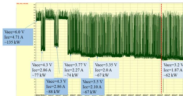
Figure 5: Power consumption of TPS BR RF system.
