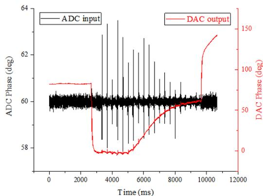
Figure 1: Phase variation of ADC and DAC of DLLRF without KPLL while beam injections.
