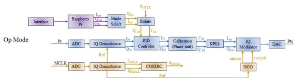
Figure 2: DLLRF architecture of the TPS.
