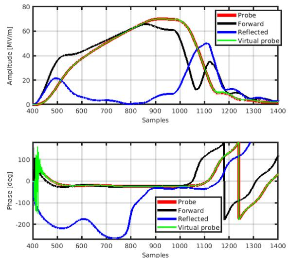
Figure 1: Calibrated signals of the ARES RF-gun in amplitude and phase for the probe, forward and reflected signal together with the virtual probe.
