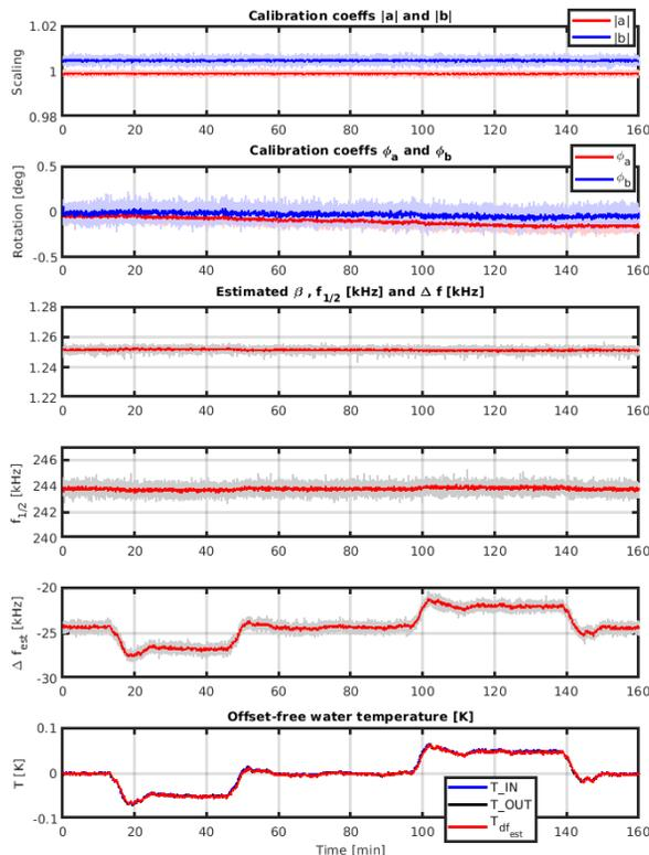
Figure 2: RF-gun temperature scan by changing the input water temperature by  $\pm 0.05$  K and keeping the drive amplitude constant. The online computed data is shown as light grey line and a moving average of 20 samples as blue and red lines for the upper plots. The last plot shows the comparison of the measured water temperature with update rate of 1 Hz and the estimated RF-gun temperature with moving average of 20 samples at 3.33 Hz to 5 Hz.
