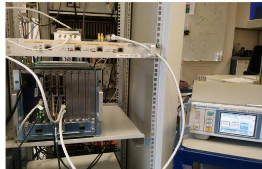
Figure 3: MTCA-Setup with X2-timers.
