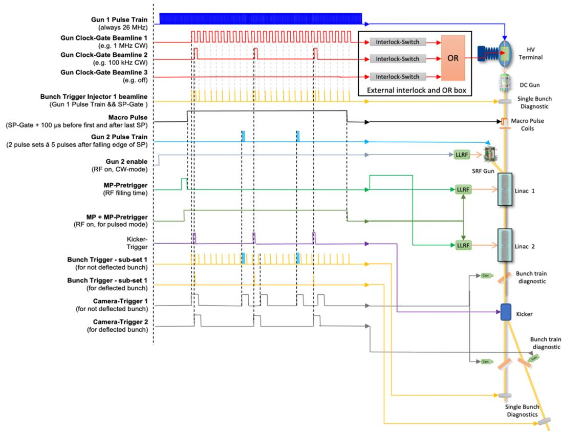
Figure 2: Example of a timing structure at ELBE using two guns and a subsequent kicker to generate complex bunch pattern.
