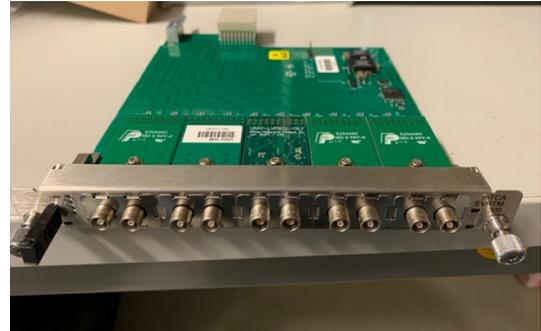
Figure 1: Micro Research Finland timing receiver rear transition board equipped with universal output modules.
