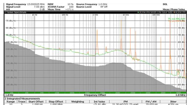
Figure 3: Output jitter performance of a TTL universal output module.
