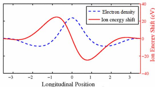
Figure 2: The electron beam density modulation due to a single proton (arb. units) and a corresponding energy kick (in eV) after the “Kicker” section as a function of the proton’s longitudinal position ( $\mu\text{m}$ ).
