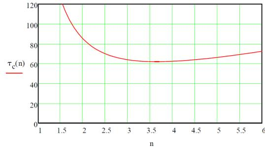
Figure 4: Cooling time (in minutes) as a function of the cooling range  $n$  defined as  $nR_{56}\delta_p = \frac{z_0}{2}$ .
