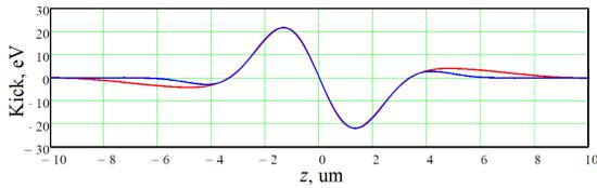
Figure 3: The energy kick (eV) after the "Kicker" section as a function of the proton's longitudinal position  $z = R_{56} \delta$  ( $\mu\text{m}$ ) with respect to the reference on-energy proton. The red curve is a calculated wake, based on [8, Eq. (C7)]. The blue curve is the proposed approximation, Eq. (1).
