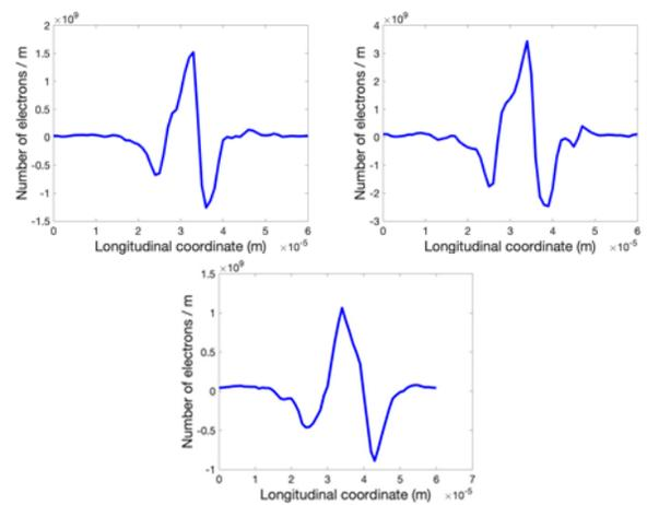
Figure 9: 1D plot of the density modulation at the entrance (top left), in the middle (top right), at the exit (bottom) of the kicker section.
