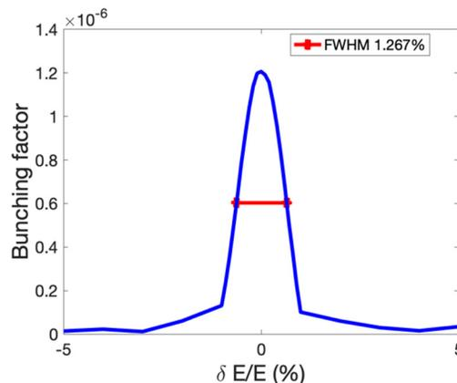
Figure 5: Bunching factor amplitude of the density modulation induced by a single ion for various energy differences between the electron beam and the ion.
