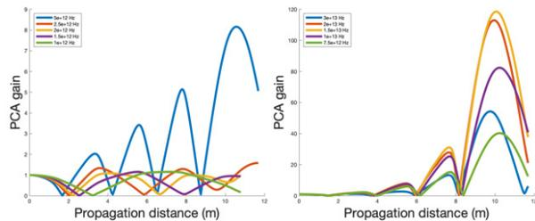
Figure 8: Evolution of PCA gain for initial density modulation at various frequencies through the PCA section.
