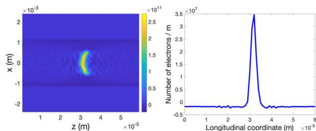
Figure 4: 2D (left) and 1D (right) plot of the density modulation in the electron beam induced by a single ion at the exit of the modulator section.
