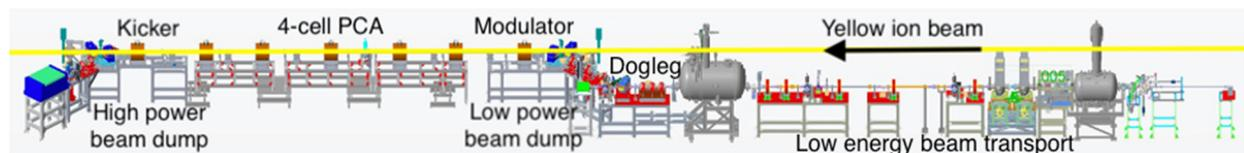
Figure 2: PCA-based CeC system installed at BNL RHIC. The electron beam is generated in a 1.25 MV superconducting radio frequency (SRF) photo-electron gun, accelerated to 14.56 MeV, and merged to co-propagate with the 26.5 GeV/u ion beam circulating in RHIC's yellow ring.
