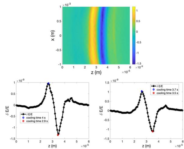
Figure 10: The energy kick to ions in the kicker section within a single pass through the PCA-based CeC system, for ions with various longitudinal and horizontal positions (top), for ions with zero horizontal position (bottom left), and for ions with horizontal offset 0.4 mm (bottom right).
