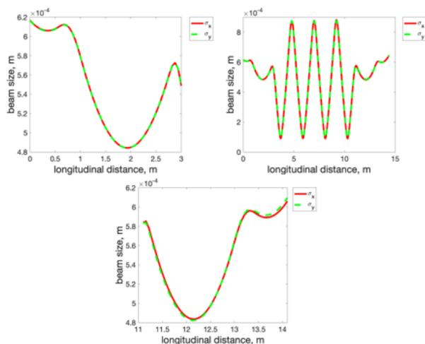
Figure 3: Evolution of transverse RMS beam size in the CeC section (top right) and the zoom-in plot for the modulator (top left) and the kicker (bottom).
