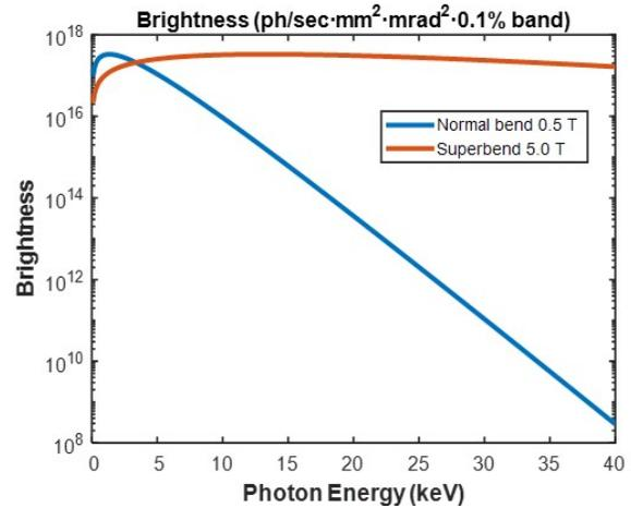
Figure 1: (left) Brightness of a SLGB (red line) versus the normal conducting bend (blue line). (right) Optimized By-field profile along the beam path by lattice design.
