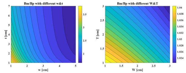
Figure 7: (left) Original MOGA optimization result of race-track type coil. (right) Load line of ( $B_p$ ) in the range of (3.8,5.0) T. The color refers to the best results of different generation ( $h=2.5$  cm,  $l=12$  cm).
