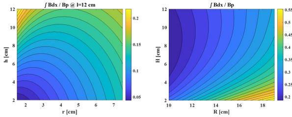
Figure 6: (left) The relative deviation between the  $|By|$ -field integral along the path from (-46,0,0.4) to (46,0,0.4) and along the standard beam path. (right) The relative deviation between the  $|By|$ -field integral along the path from (-46,0.4,0) to (46,0.4,0). The coordinate unit here is cm.
