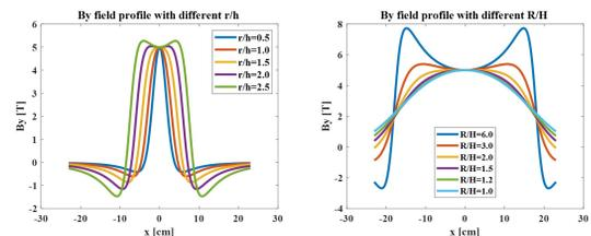
Figure 5: (left) The maximum B-field in the racetrack-type coil changes with  $w$  &  $t$  ( $r=1.5$  cm,  $l=12$  cm). (right) The B-field generated by solenoid coil at the maximum B-field point in racetrack-type coil changes with  $W$  &  $T$ .  $(r, w, h, t, l)=(1.5, 3, 2.5, 5, 12)$  cm is chosen for the solenoid coil and  $R=18$  cm,  $H = h + t - T$ .
