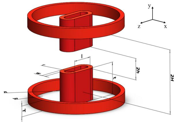
Figure 2: (left) Geometric parameters of race-track coil and solenoid coil,  $(r, w, h, t)$  for race-track coil and  $(R, W, H, T)$  for solenoid coil. (right) NbTi critical current density from WSTC (measured and fitted).
