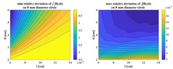
Figure 8: Original MOGA optimization result of SLGB composed of race-track type coil and solenoid coil ( $h=2.5$  cm,  $l=12$  cm).
