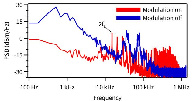
Figure 3: Spectra of the pulse amplitude evolution with (red) and without (blue) modulation. The spectra were calculated by a FFT for the time ranges 40 ms to 100 ms and 140 ms to 200 ms of Fig. 2.
