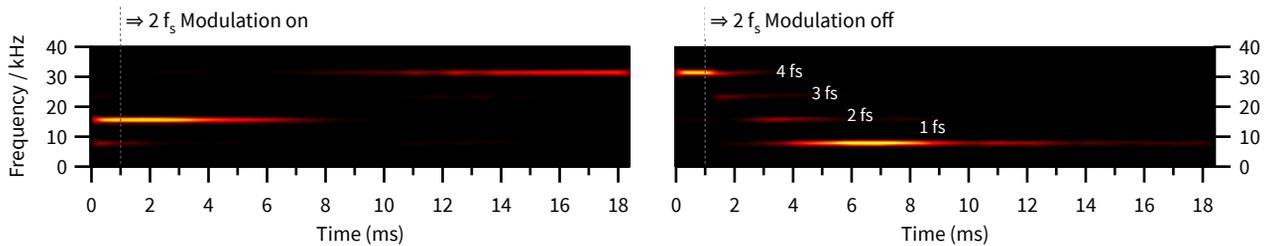
Figure 5: Wigner transform of the APD amplitude evolution. Due to an aperture, the APD amplitude is sensitive to the bunch position. Without modulation, only the synchrotron frequency is seen. When switching the modulation on, a strong 2fs line is seen for a short time, then 4fs becomes dominant.
