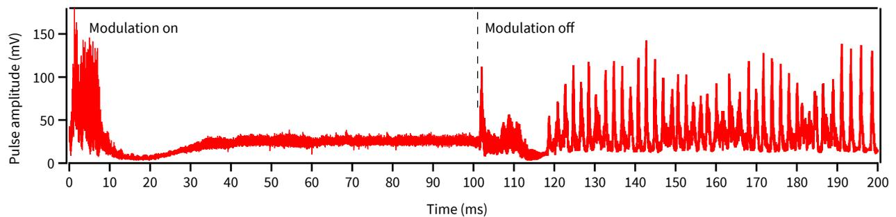
Figure 2: Influence of 2fs RF phase modulation on the bursting behavior. Pulse amplitude of a broadband THz detector read out by KAPTURE. The modulation is turned on 1 ms after the start of the measurement and turned off 100 ms later. The width of the line is caused by high frequency oscillations, which cannot be resolved in the shown time scale.
