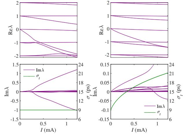
Figure 2: Effect of bunch lengthening on the frequencies (top) and damping/growth rates (bottom) of the 10 lowest vertical modes.
