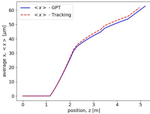
Figure 3: Center of mass transverse displacement induced by a misaligned section ( $\Delta x_2 = 50 \mu\text{m}$ ,  $\delta_2 = 50 \mu\text{rad}$ ).
