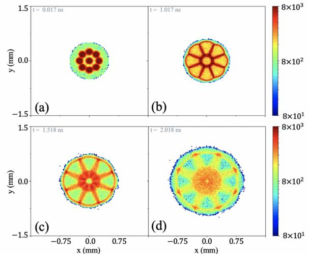
Figure 4: Time evolution of nine beamlets spatially scaled down by 50%. Plotted is the charge density ( $\mu\text{C}/\text{m}^3$ ) at time  $t=0$  ns (a), 1 ns (b), 1.5 ns (c) and 3 ns (d).
