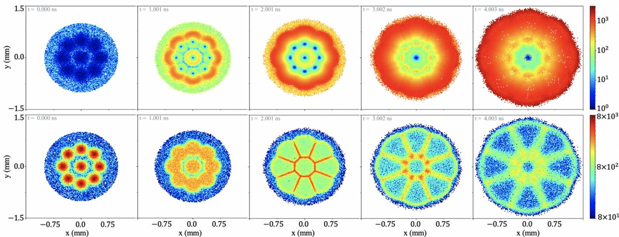
Figure 1: Time evolution of nine beamlets initially at 1 K with an electron halo initially at 10 K. Plotted is the electron temperature (K) above and charge density ( $\mu\text{C}/\text{m}^3$ ) below at time  $t=0$  ns, 1 ns, 2 ns, 3 ns, and 4 ns from left to right.
