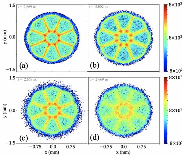
Figure 2: Charge density ( $\mu\text{C}/\text{m}^3$ ) after 3 ns for variations of initial beamlet and halo temperatures:  $T_b = T_h = 0.2$  mK (a),  $T_b = 1$  K and  $T_h = 10$  K (b),  $T_b = 10$  K and  $T_h = 100$  K (c),  $T_b = 100$  K and  $T_h = 10$  K (d).
