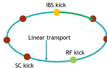
Figure 1: Schematic of PyHEADTAIL simulation structure.
