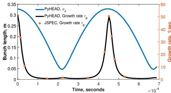
Figure 3: Bunch length and longitudinal growth rate evolution during bunch rotation process.
