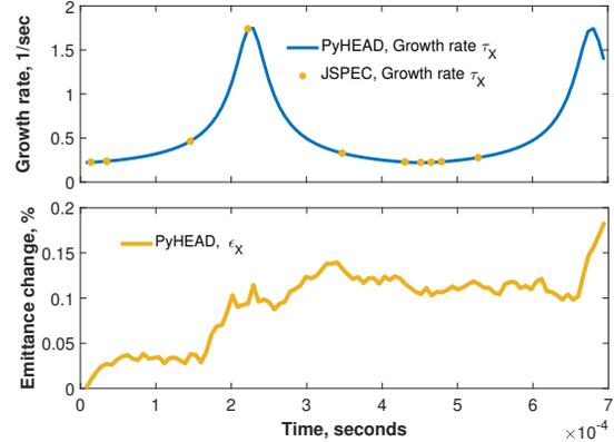
Figure 4: (Top) horizontal growth rate  $\tau_x$  and (bottom) horizontal rms emittance  $\epsilon_x$  evolution during bunch rotation.
