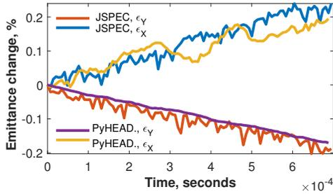
Figure 2: Comparison of transverse rms emittance evolution between JSPEC and PyHEADTAIL.
