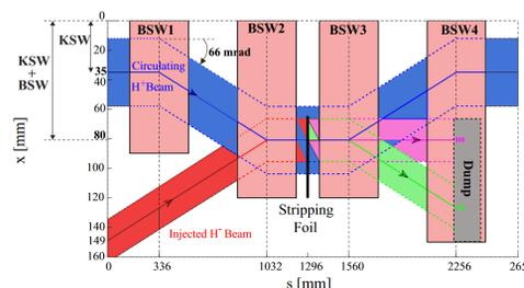
Figure 1: Schematic of the PSB H<sup>-</sup> injection system [1].
