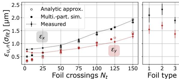
Figure 3: Left: Transverse emittances for varying number of foil hits  $N_t$ , foil type 3. Right: Different foil types,  $N_t = 150$ .
