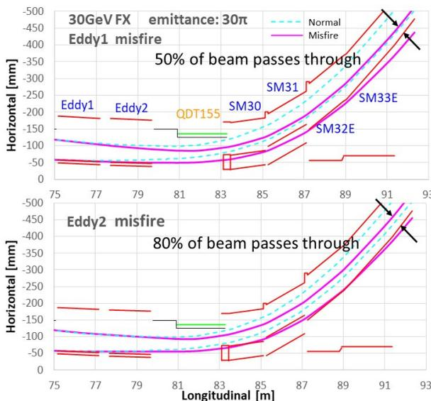
Figure 4: Simulation of the eddy SM failure.
