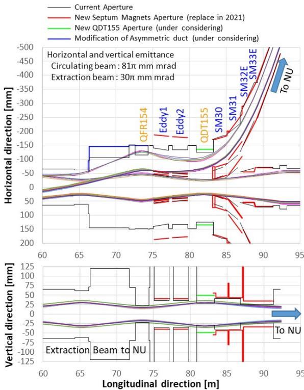
Figure 3: New Aperture plans and beam envelopes.
