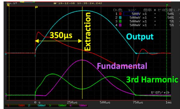
Figure 5: Pulse operation of the eddy SM.
