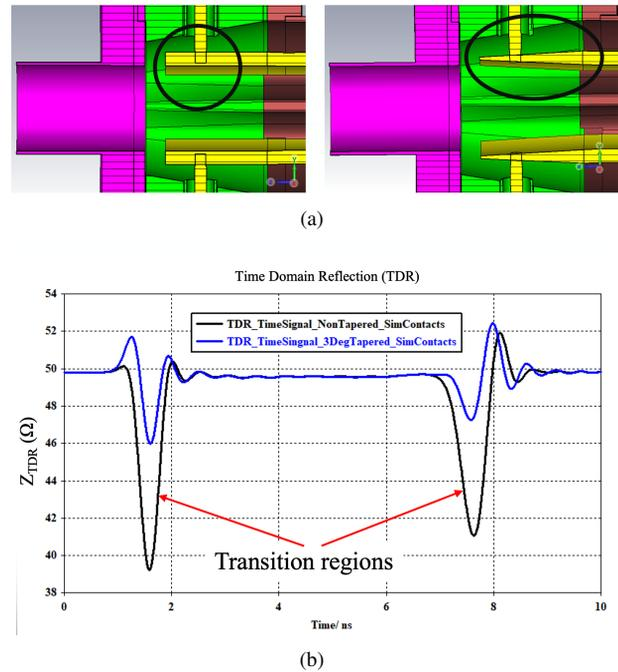
Figure 3: (a) CAD design showing the non-tapered (left) and tapered electrodes (right). (b) TDR plot comparison between the non-tapered (black curve) and tapered (dark blue curve) electrodes.
