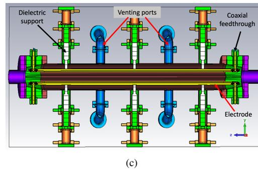
Figure 1: (a) Cross-section of the kicker with curved (left) and half-moon (right) electrodes, (b) comparison of electric fields produced by the curved and half-moon (flat) electrodes respectively, where the solid and dashed curves represent curved and flat electrodes respectively, and (c) plain view of the injection kicker geometry with dielectric supports and pumping ports in the middle.
