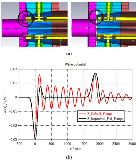
Figure 2: (a) CAD model of the injection kicker with (left) and without deep pockets (right) in the end-flange. (b) Wakefield comparison between these two geometries.
