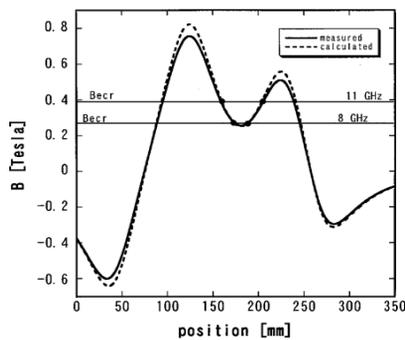
Figure 2: Magnetic field profile of the ECR ion source.
