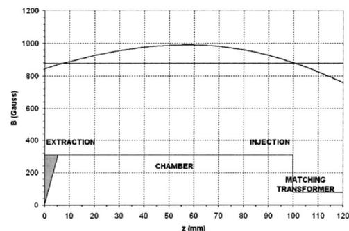
Figure 1: The most optimal magnetic field profile of a microwave discharge ion source. The stable line depicts the resonance magnetic field at the frequency of 2.45 GHz.
