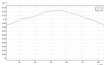
Figure 7: Axial magnetic field profile of the microwave source operating mode with the fixed position of the ring magnets.
