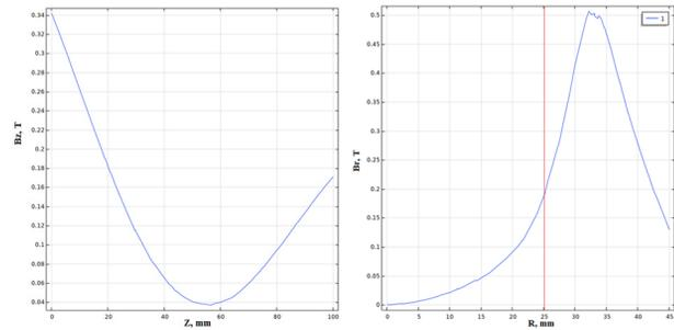
Figure 4: Axial and radial magnetic field profiles of the optimized magnetic system configuration.
