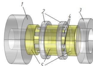
Figure 5: The model of the magnetic system modification with three solenoids. (1) Injection ring magnet. (2) Middle ring magnet. (3) Extraction ring magnet. (4) Hexapole magnet. (5) Solenoids.
