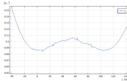
Figure 8: Axial magnetic field profile of the microwave source operating mode with the adjustable position of the ring magnets.
