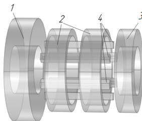
Figure 3: The magnetic system of the 2.45 GHz ECRIS. (1) Injection ring magnet. (2) Middle ring magnet. (3) Extraction ring magnet. (4) Hexapole magnet.
