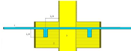
Figure 1: 40 kV DC break design with PTFE. (1) Insulator. (2) Waveguide flange. (3) WR340 waveguide.
