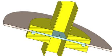
Figure 3: 40 kV DC break design with composite dielectric. (1) Alumina. (2) PTFE.
