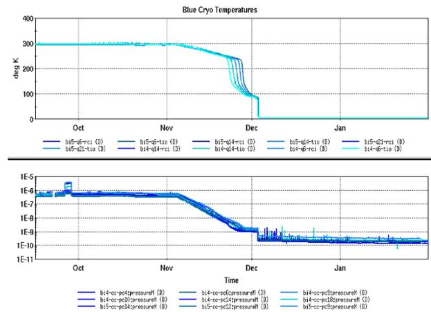
Figure 3: Vacuum as a function of the magnet temperature during cooldown prior to a recent RHIC run.
