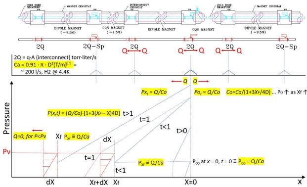
Figure 4: Sketch of the 1-D wave propagation model for one section of a EIC superconducting arc.
