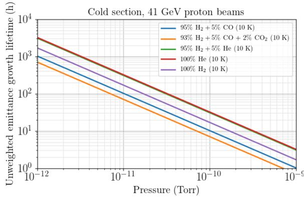
Figure 2: Unweighted emittance growth lifetime for the 41 GeV proton beam in the cold section of RHIC versus pressure.
