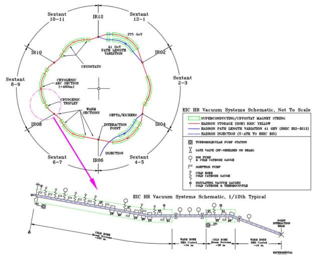
Figure 1: Sketch of the EIC hadron beamline system.
