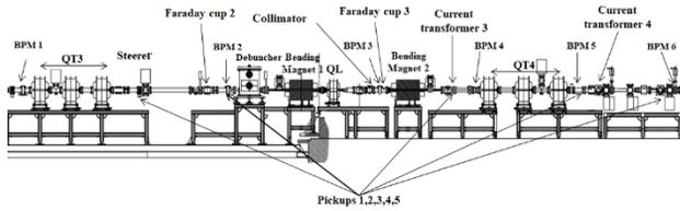
Fig. 8: Beam diagnostic units arranged along HEBT.
