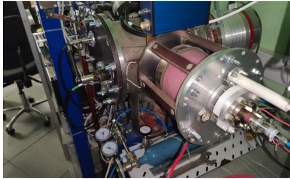
Figure 3: Helium ion source at the test bench.
