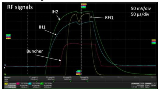
Fig. 10: RF dropdowns in the HILAC cavities.
