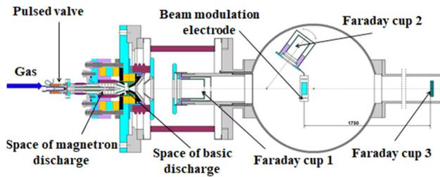
Figure 2: Test bench layout for the TOF measurements.
