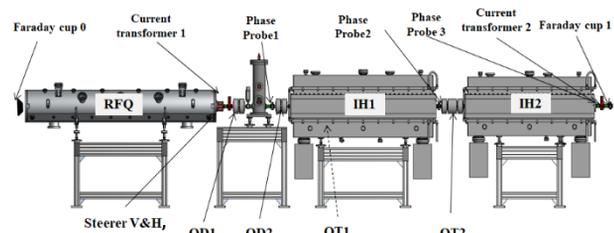
Fig. 7: Beam diagnostic units arranged along HILAC.
