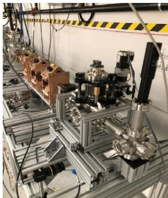
Figure 9: Beam halo monitor installed at AWA beamline.
