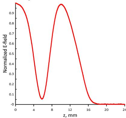
Figure 5: Bead pull measurement result at 11.7 GHz.
