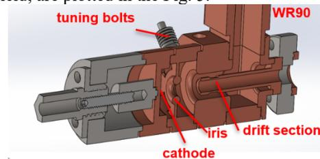
Figure 1: Engineering design of UHGPI.
