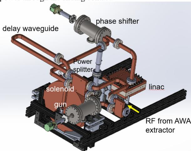
Figure 9: RF transmission line feeding gun and linac.
