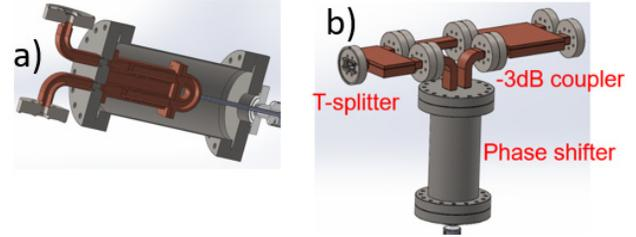
Figure 10: Broadband RF components: a – phase shifter, b – power splitter.
