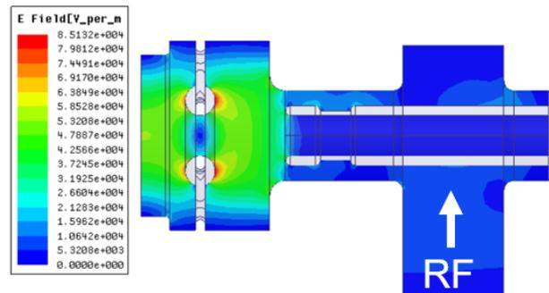
Figure 2: Field structure in gun at 11.7 GHz.
