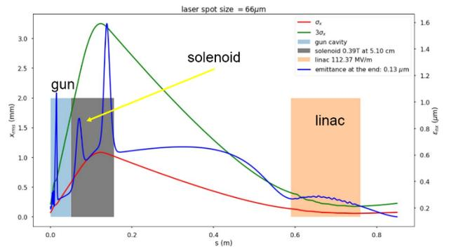
Figure 7: Evolution of the RMS beam size (red) and emittance (blue) along gun beamline.
