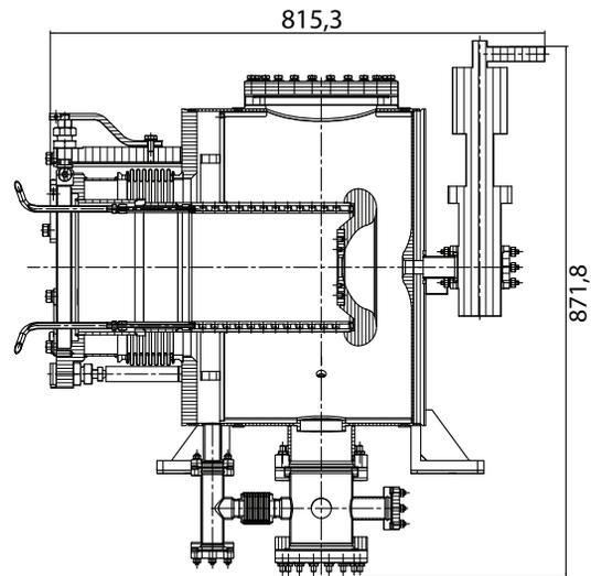
Figure 2: Structural drawing of the RF gun.
