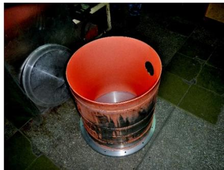
Figure 6: Outer stainless-steel cylinder covered by copper metal.
