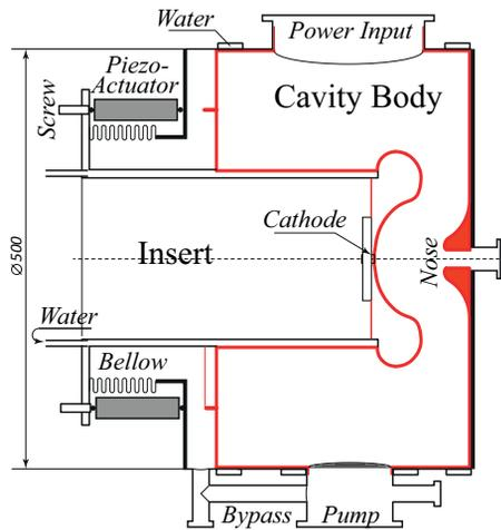
Figure 1: Schematic view of the RF gun.
