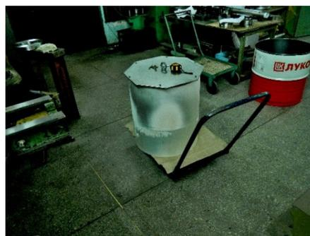
Figure 7: Inner copper cylinder covered by argenta metal.
