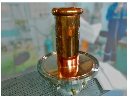
Figure 4: Example of the beam welding of the Insert with the cavity wall [3].
