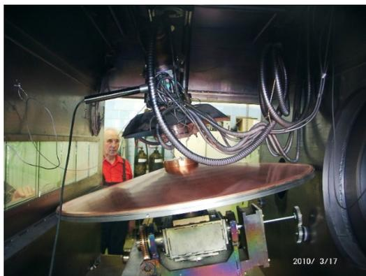
Figure 3: Example of the beam welding of the cavity wall center with the Nose [2] (that is shielded by a cover).
