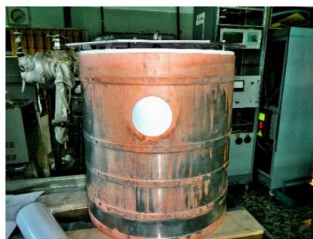
Figure 8: Inner copper cylinder, after its cooling by liquid nitrogen, is inserted into the outer cylinder.
