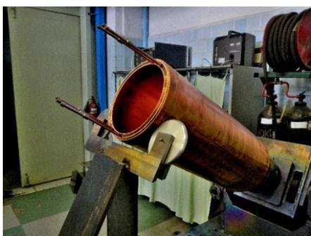
Figure 5: Example of the beam welding of Insert edges for water channels [2].
