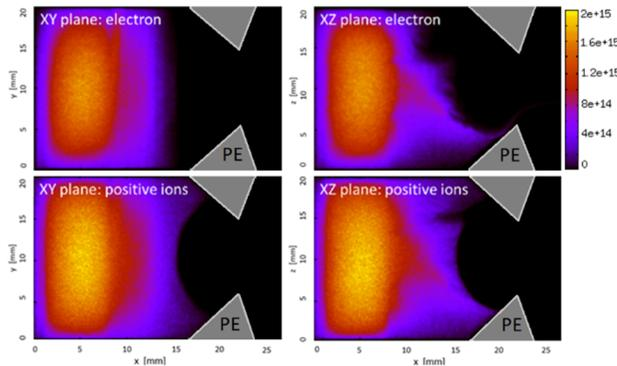
Figure 4: Density maps of electron (top) and positively charged particles ( $H^+$ ,  $H_2^+$ ,  $H_3^+$ ) (bottom) in the ( $x$ - $y$ ) (left) plane and ( $x$ - $z$ ) (right) plane where filter field generated asymmetry is clearly visible.
