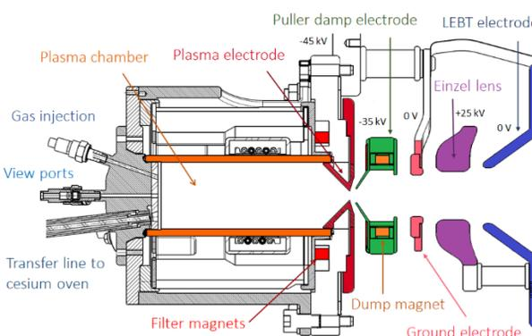
Figure 1: IS03b Linac4 H<sup>-</sup> ion source and extraction system. This source operates in volume and plasma surface H<sup>-</sup> production modes.
