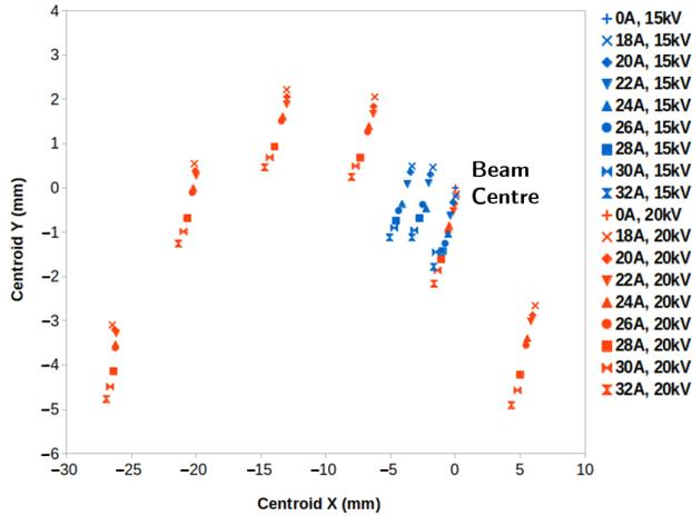
Figure 6: The  $x$  and  $y$  position of the centroids of the beam spots imaged with the Setup 1 (blue) and Setup 2 (red) with increasing magnetic field strength.
