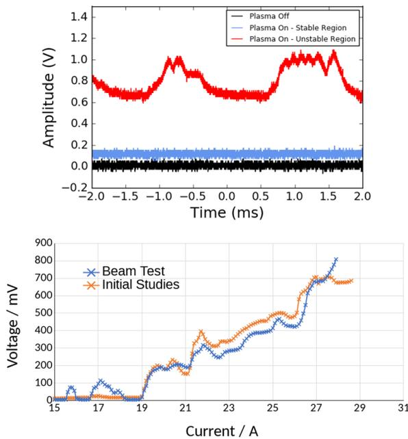
Figure 3: Top—Variation of discharge current from the lens in three regions: plasma off, plasma on, and plasma on in unstable region. Bottom—Voltage-current characteristic of the lens on the beam line (blue crosses) compared to measurements in the laboratory at ICL (orange crosses).
