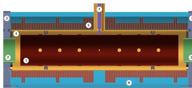
Figure 1: Internal structure of the ICL Gabor lens (longitudinal cross-section). The main components are: 1-central anode, 2-end electrodes, 3-end flanges, 4-vacuum tube, 5-pancake coils, 6-outer tube, 7-high-voltage feed-through.
