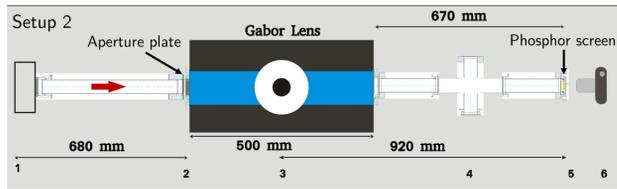
Figure 2: Schematic of the day 2 beam test setup. A different setup with a beam pipe of only 380 mm upstream of the lens was used in day 1 of the beam test.
