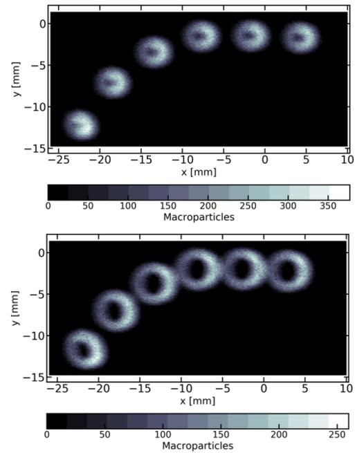
Figure 8: The effect of a plasma column rotating around the beam axis on six proton pencil beams as simulated with BDSIM [8] for electron densities of  $0 \text{ m}^{-3}$ ,  $1.8 \times 10^{13} \text{ m}^{-3}$ , and  $2.8 \times 10^{14} \text{ m}^{-3}$ . The uniform plasma column had a radius of 14 mm and it was displaced off-axis by 7 mm.
