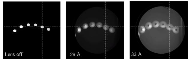
Figure 4: Camera image of the 6 beam spots beyond the aperture with a lens voltage of 20 kV and a current through the coils of 0 A, 28 A, and 33 A. The dashed lines indicate the beam axis.
