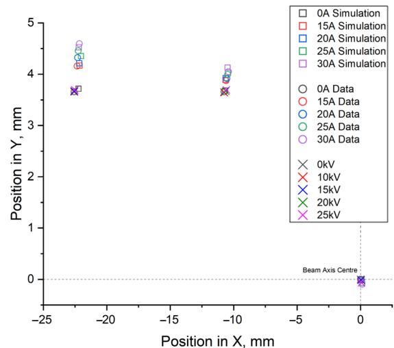
Figure 5: Position of the centroid of 3 beam spots. Squares and Circles represent variation in current through the coils only with no applied high voltage. Crosses represent variation in high voltage with no current through the coils.
