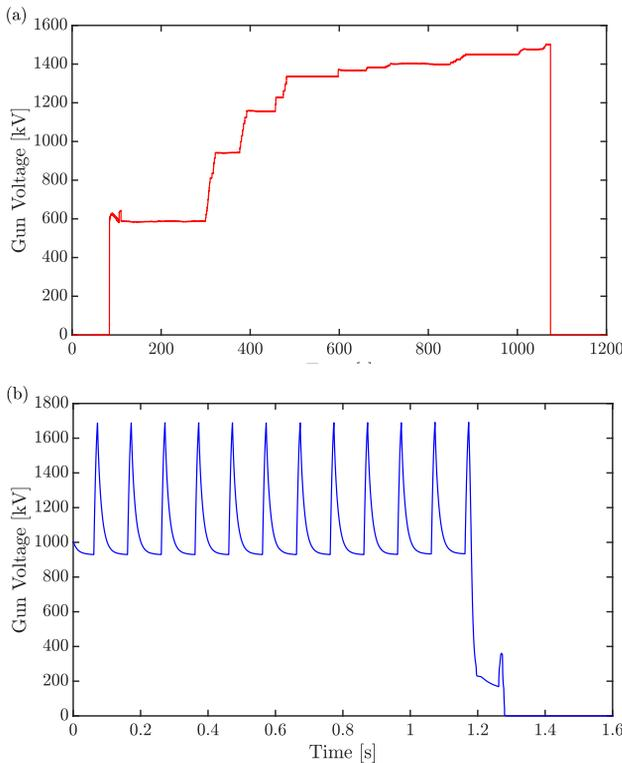
Figure 1: Maximal achieved cavity voltage in CW (a) and pulsed (b) modes after the gun conditioning.
