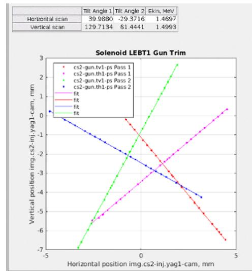
Figure 2: Energy measurement using dark current shows the achieved voltage of 1.5 MV CW.
