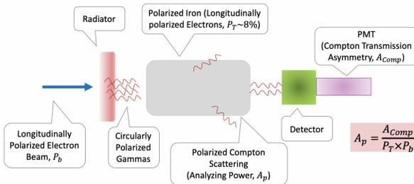
Figure 4: Schematic of the Compton polarimeter.
