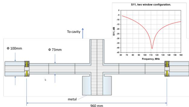
Figure 3: An example of the antenna configuration utilizing two windows with 50 kW CW per window.
