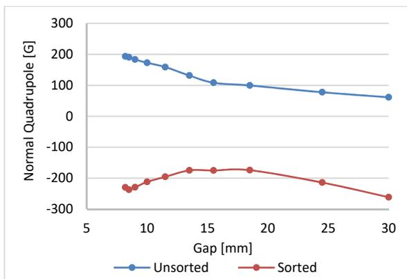
Figure 1: Comparison of normal quadrupole components with  $M_x$  sorted and unsorted for the APS27#3 device (a 27-mm-period undulator).
