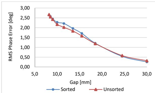
Figure 5: Comparison of RMS phase errors vs. gap for the APS28#13S undulator with sorted and unsorted magnets after final tuning. The RMS phase error requirement for the APS-U is less than  $3^\circ$ .
