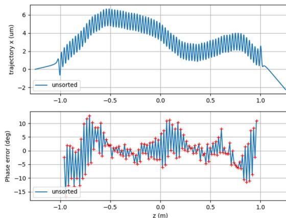
Figure 3: Computed as-assembled trajectory at 6 GeV (top) and RMS phase errors (bottom) before tuning for the unsorted case for APS28#13S undulator at 8.2-mm gap. The as-assembled RMS phase error was  $5.51^\circ$ .
