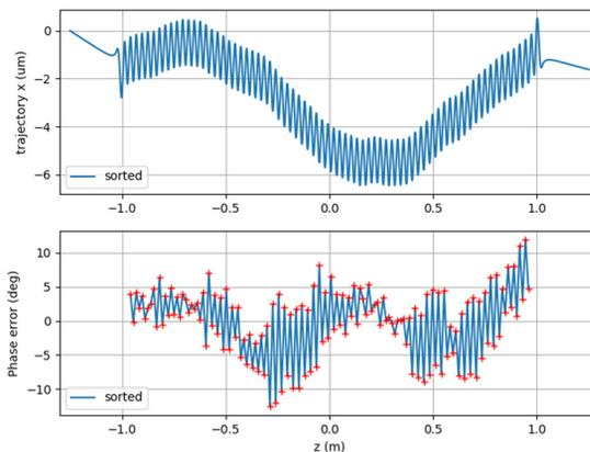
Figure 2: Computed as-assembled trajectory at 6 GeV (top) and RMS phase errors (bottom) before tuning for the sorted case for the APS28#13S undulator at 8.2-mm gap. The as-assembled RMS phase error was  $4.88^\circ$ .
