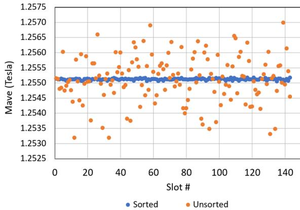
Figure 4: Average top-bottom jaw total moment distribution of device APS28#13S for sorted and unsorted cases. The RMS value is  $2.54 \times 10^{-5}$  Tesla for the sorted case and  $7.73 \times 10^{-4}$  Tesla for the unsorted case.
