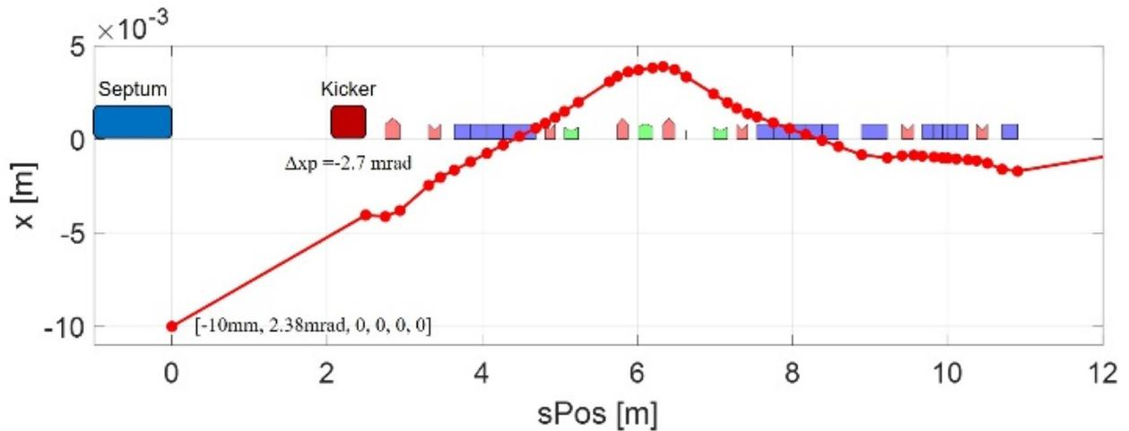
Figure 6: First turn trajectory of the injected particle and specific parameters of the injection scheme.
