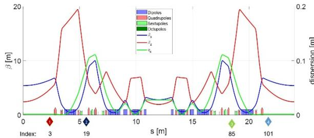
Figure 2: Lattice functions of the HALF 2.2 GeV storage ring and four possible positions to install kicker.
