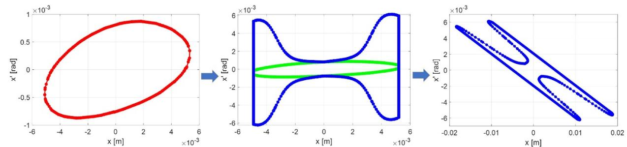
Figure 4: Acceptance at positions of nonlinear kicker and the injection point in scheme 1.
