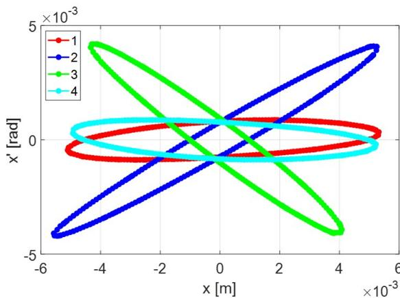
Figure 3: Comparison of the acceptance at different positions.
