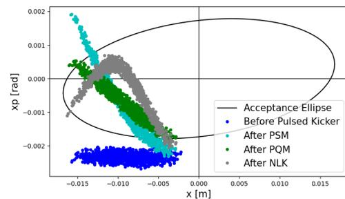
Figure 3: Beam distribution in horizontal phase space before and after a single kick from each alternate injection scheme. In each case a 30 cm magnet is placed at  $s = 29.2165$  m, the end of the third straight section.
