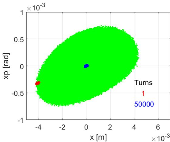
Figure 6: Simulation result of the betatron oscillation.
