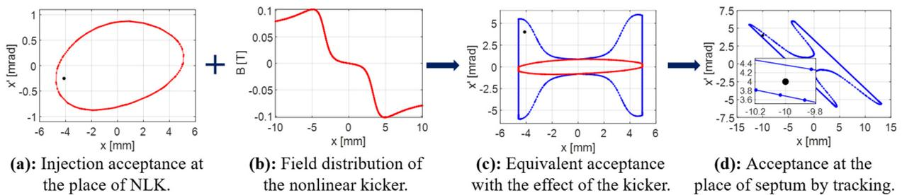
Figure 3: The progress of acceptance analysis.
