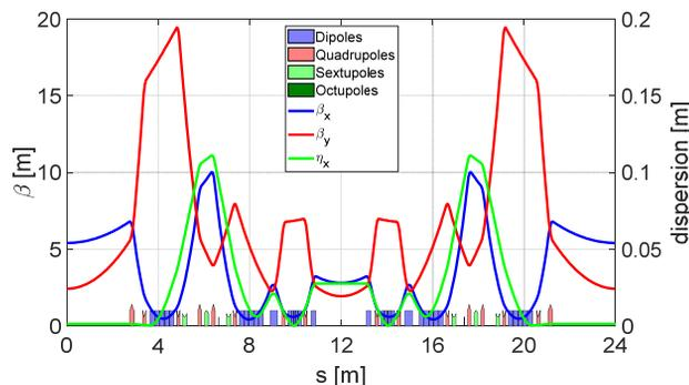
Figure 1: Magnet layout and linear optical functions.
