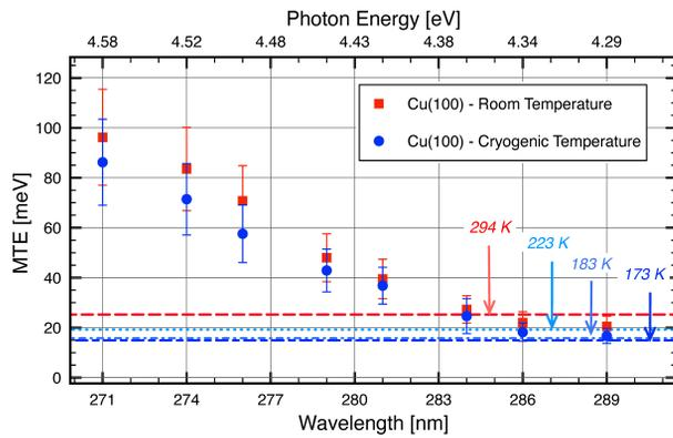
Figure 2: MTE values for a single crystal Copper (100) cathode at two different temperatures. The energy limit at different temperatures is shown by dotted lines.
