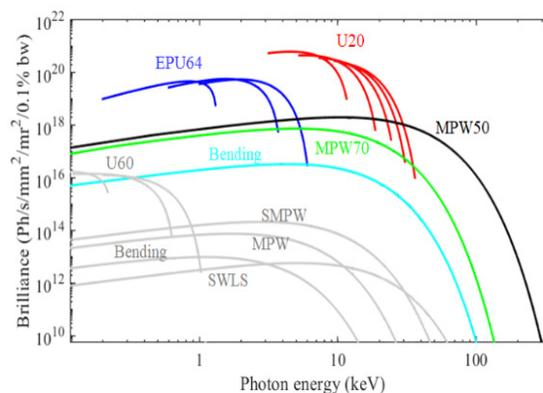
Figure 1: Brilliance of synchrotron light radiated as a function of photon energy from the existing 1.2 GeV machine (grey) and SPS-II (color).
