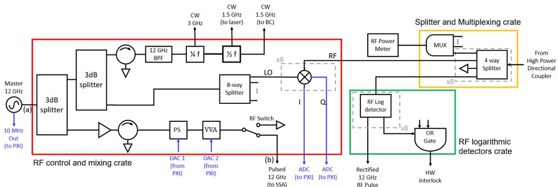
Figure 1: Simplified diagram of the Low Level RF System layout. The three coloured boxes define the three crates. Blue arrows define signals which are sent to the PXI control system.
