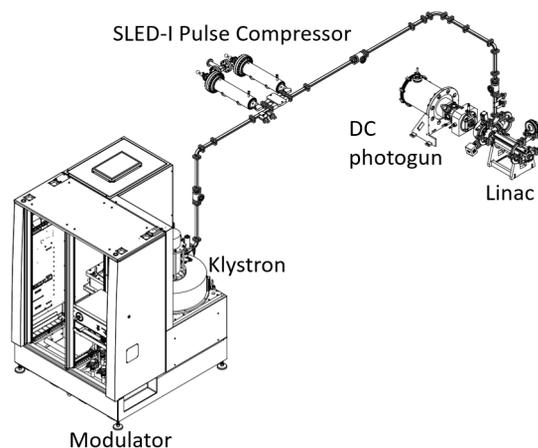
Figure 3: High Power RF Network.
