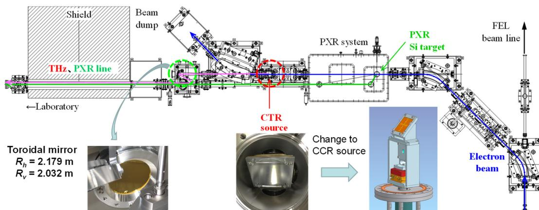
Figure 3: Schematic layout of CCR-MCP in the PXR section at LEBRA.
