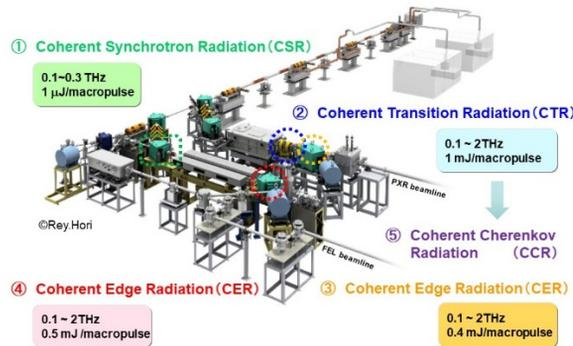
Figure 1: Schematic view of coherent radiation sources at LEBRA.
