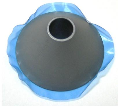
Figure 4: Photograph of the hollow conical made of HR silicon.
