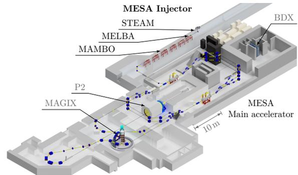
Figure 1: MESA operating parameters  $f = 1.3 \text{ GHz}$ ,  $E_{\text{EB}} = 155 \text{ MeV}$  |  $E_{\text{ER}} = 105 \text{ MeV}$ ,  $I_{\text{EB}} = 150 \mu\text{A}$  |  $I_{\text{ER}} = 1 \text{ mA}$ .
