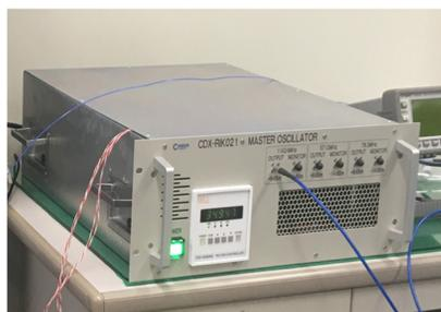
Figure 4: RF master oscillator.
