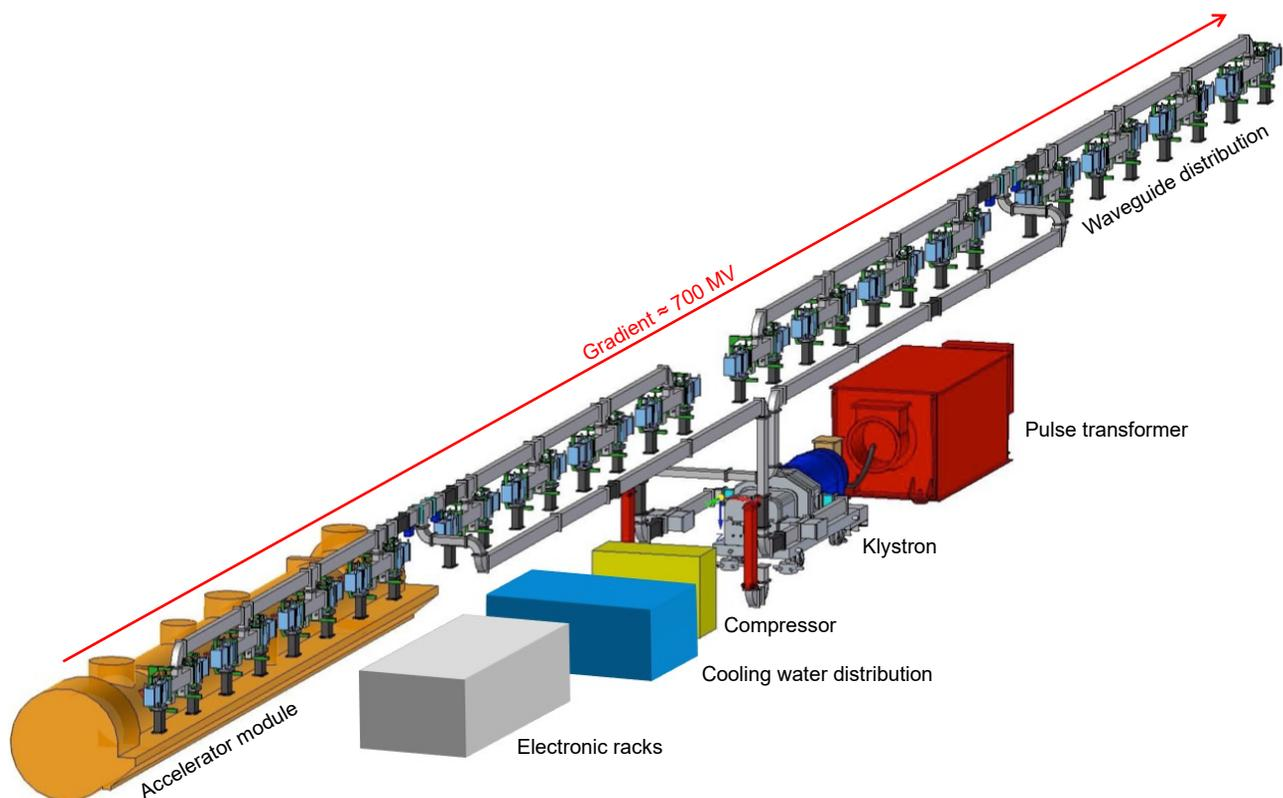
Figure 2: One RF station in the accelerator tunnel.
