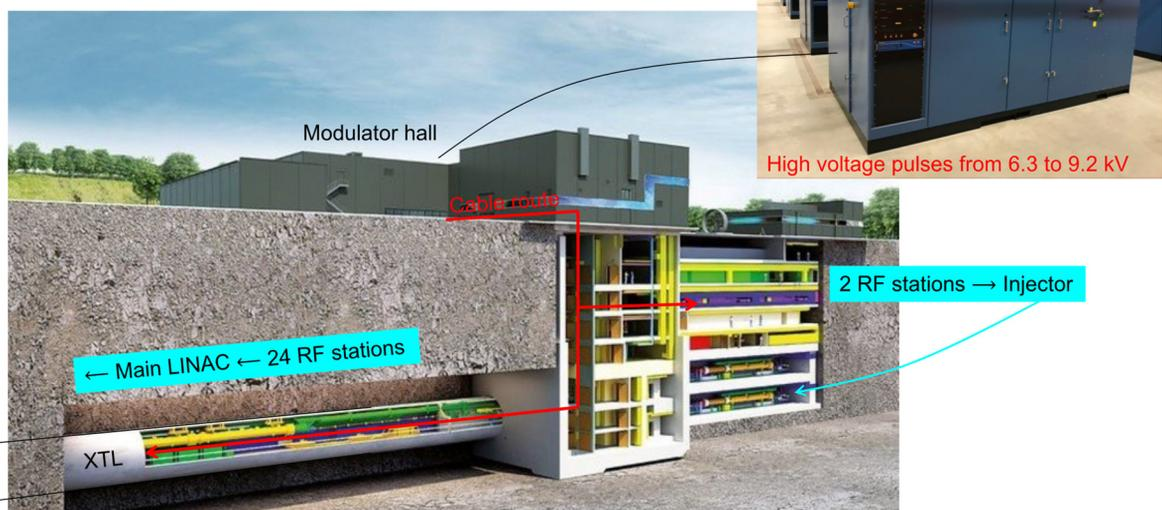
Figure 1: Hall with 26 modulators and cable routes for the high-voltage pulses to the RF stations.
