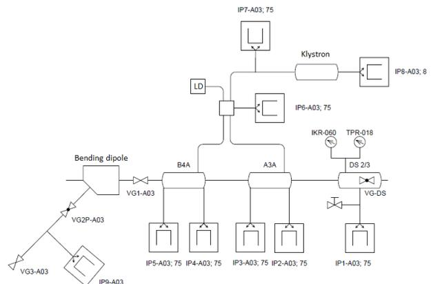
Figure 2: Vacuum system layout of one linac station.
