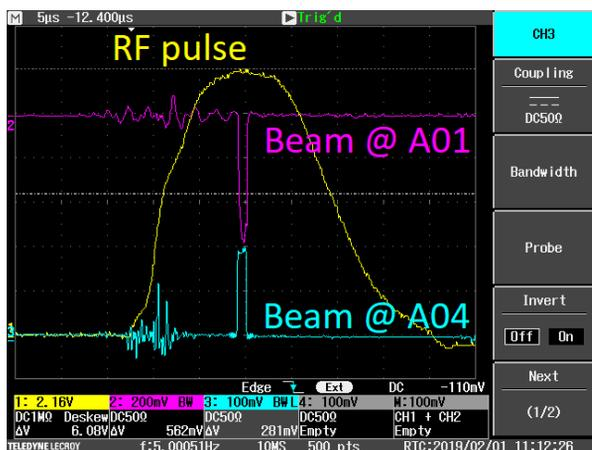
Figure 3: Beam current signal from the current transformer after A01 (magenta) and A04 (cyan) stations, and RF pulse (yellow).
