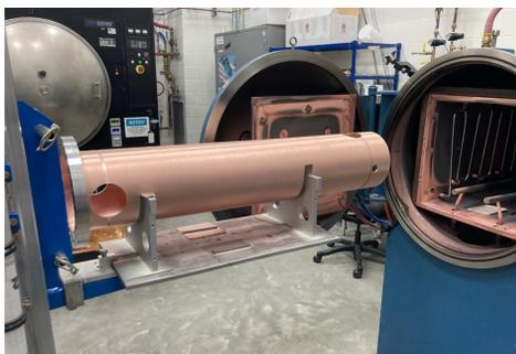
Figure 4: The harmonic kicker prototype in fabrication.
