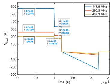
(b) The forward voltage on  $50 \Omega$  transmission line.
