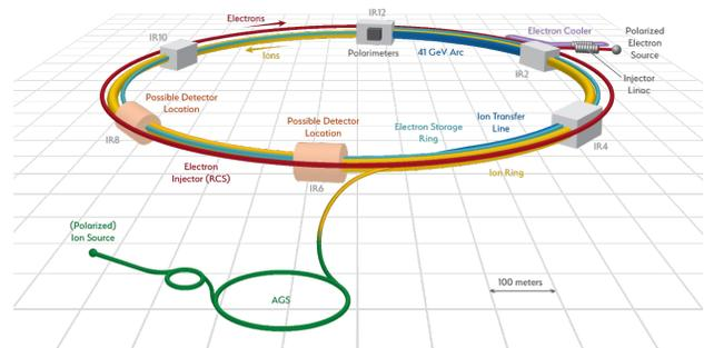
Figure 1: Schematic diagram of the EIC layout.
