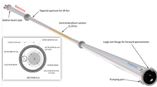
Figure 3: Beampipe for the EIC IR.
