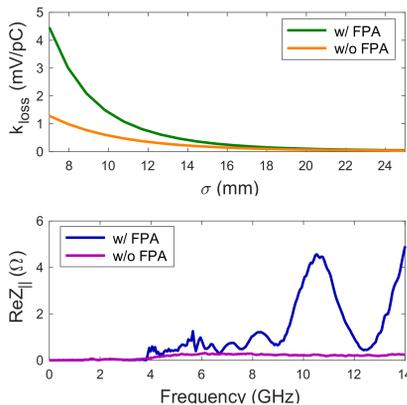
Figure 4: Impedance of the electron beam pipe.
