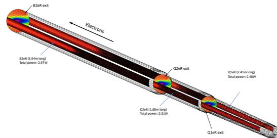
Figure 5: Anticipated synchrotron radiation power deposition on the rear-side beam pipes.
