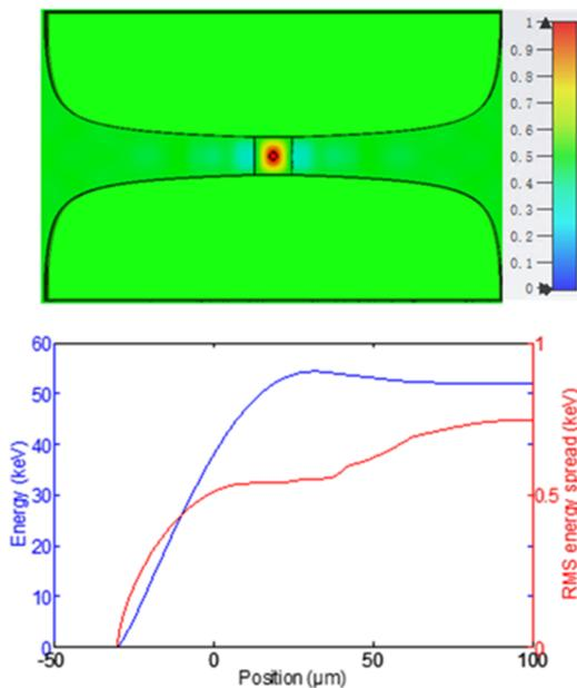
Figure 2: Simulated electric field and the beam energy.
