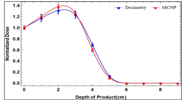
Figure 3: Depth-dose distribution inside the PP dummy irradiated by UELR-10-15S2 accelerator.
