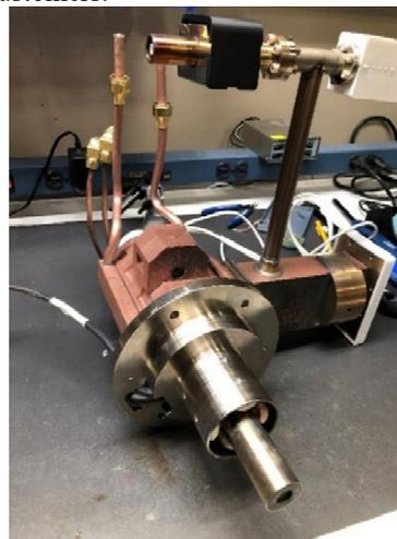
Figure 1: ABC-3-S-X IN004 prototype fully tuned and sealed under ultra-high vacuum.
